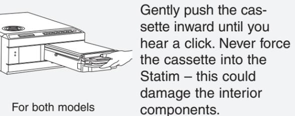
Gently push the cassette inward until you hear a click. Never force the cassette into the Statim – this could damage the interior components.
